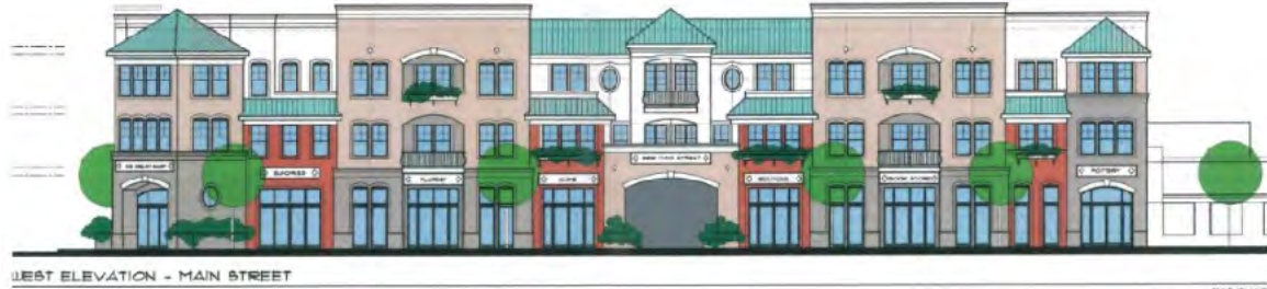
Figure 2: Example of block front elevation with horizontal and vertical offsets to add visual interest.
